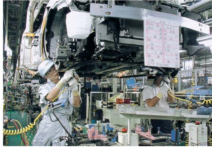
Assembly line workers install a hybrid engine in a Toyota sedan
